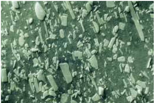
SiC particles in a Si 3 N 4 matrix , 1000X (DIC)
