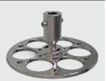
FEMTO-1100S individual specimen holder, requires 6 plastic rings ranging from 1-inch up to 1.5-inch or 25 mm up to 40 mm (ordered separately) Catalog no. SH-1100
