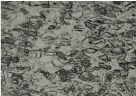
99.9% Silver, etched with ammonia peroxide, 200X B.F.
