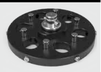
Central 1-inch or 25 mm specimen holder for FEMTO-1500S Catalog no. QRC-SH100A-1500
