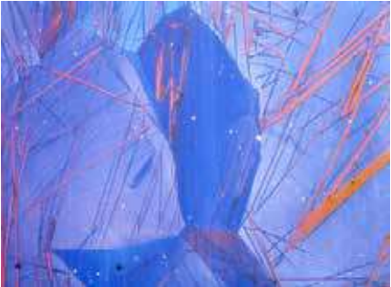
Fe-Ni-Co-Al Alloy, 400X (Polarized Light)
